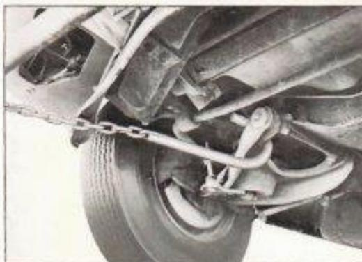
Fig. 3—Place Hooks through Lower Control Arms
