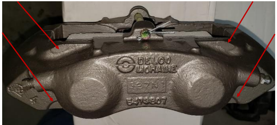
Fig. #1. RF Caliper side. Red arrows show semi-circles that were spot faced, leaving no paint.
